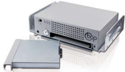
BOP HD: 400 frames per second (global frame rate) BOP EQ: 200 frames per second (global frame rate) Secure removable Slidedisk hard drives
